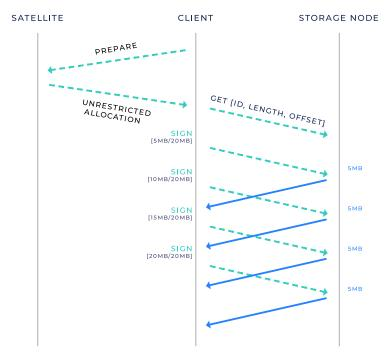
Figure 4.6: Diagram of a get operation
