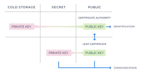
Figure 4.3: The different keys and certificates that compose a storage node's overall identity. Each row represents a private/public key pair.
