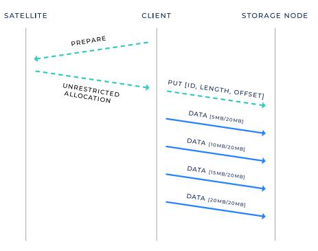
Figure 4.5: Diagram of a put operation
